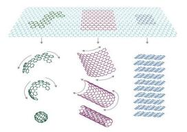
Figure 2. Graphene (top) and associated structures: fullerene (bottom left); carbon nanotubes (bottom centre); and graphite (bottom right).
