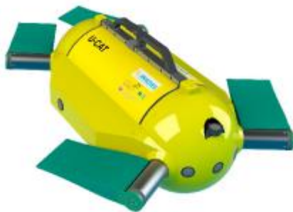
The biomimetic AUV U-CAT
