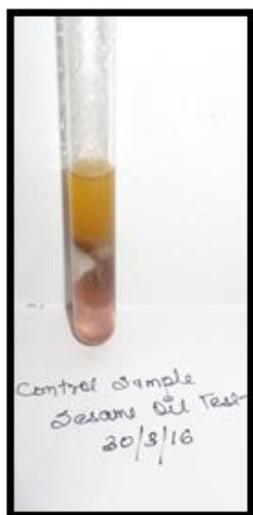
Figure – 4.10. Positive test of sesame oil showing pink colour, 4.11. Negative test of sesame oil showing no colour
