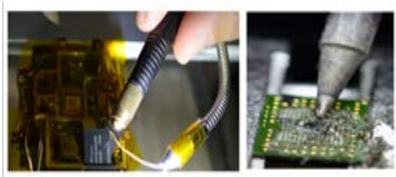
Figure No. 1: Chip off Technology
