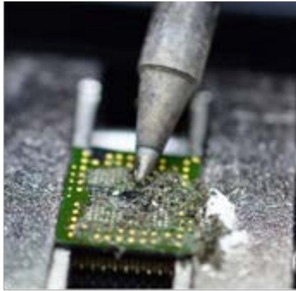
Figure No. 4: Heating Compound with Solder
