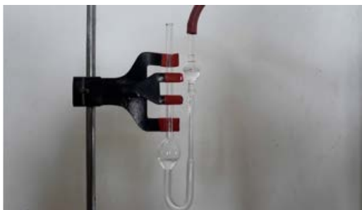
Figure No. 2: Viscometer to show the detection of Viscosity
