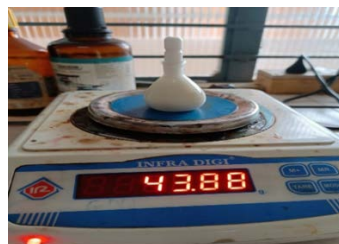
Figure No. 1: specific gravity bottle for the detection of density
