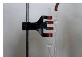
Figure No. 2: Ostwald's Viscometer for measuring Viscosity
