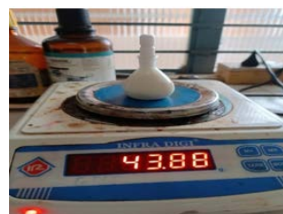
Figure No. 1: Specific gravity bottle for measuring density
