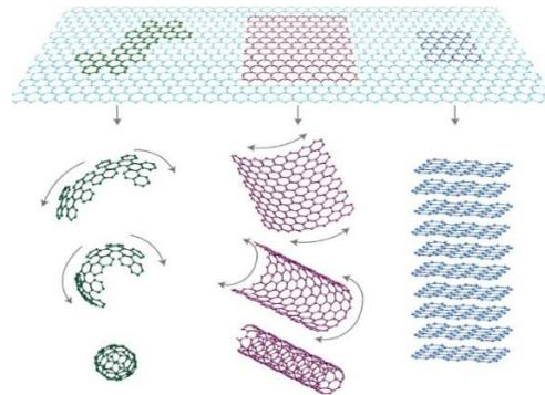
Figure 2. Graphene (top) and associated structures: fullerene (bottom left); carbon nanotubes (bottom centre); and graphite (bottom right).
