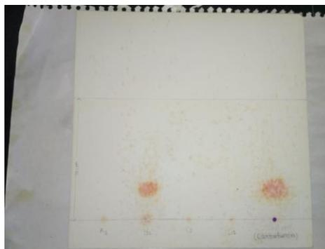
**Figure No. 7 – TLC Plate of Fruits Sample with standard Carbofuran**
