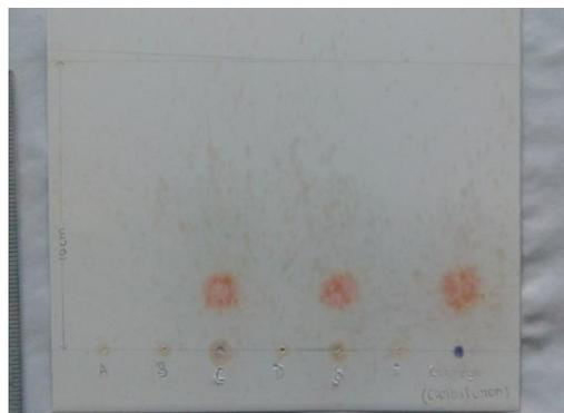
**Figure No. 4 – TLC Plate of Vegetable Sample with standard Carbofuran**
