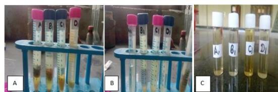
Figure No. 2 – Pesticide Residue Extraction from Fruit Samples: A) Homogenized Fruit Samples for Pesticide Residue Extraction, B) Pesticide Residue Extract of Fruit Sample, C) Pesticide Residue Extract of Fruit Sample after cleanup
