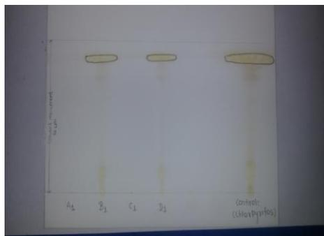
**Figure No. 6 – TLC Plate of Fruits Sample with standard Chlorpyrifos**
