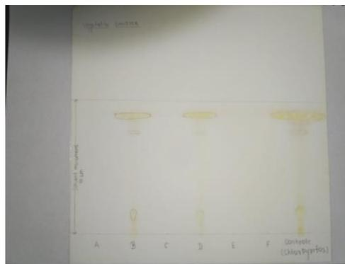
**Figure No. 3 – TLC Plate of Vegetable Sample with standard Chlorpyrifos**
