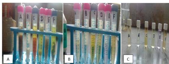
Figure No. 1 – Pesticide Residue Extraction from Vegetable Samples: A) Homogenized Vegetable Samples for Pesticide Residue Extraction, B) Pesticide Residue Extract of Vegetable Sample, C) Pesticide Residue Extract of Vegetable Sample after cleanup.
