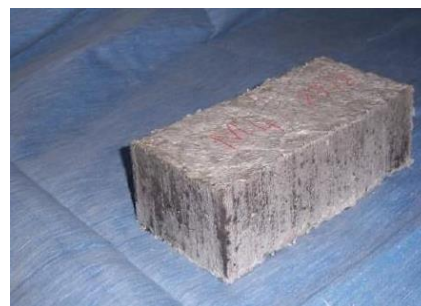
Figure 3: Prepared Papercrete Brick (Shermale and Varma, 2015)
